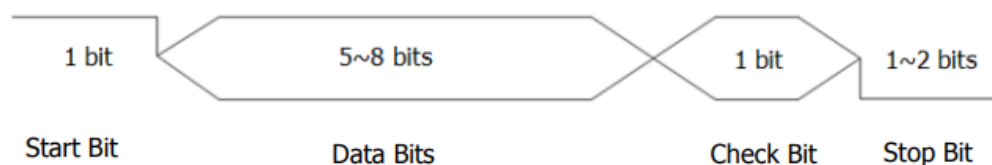
Figure 8.9 Schematic Diagram of UART Protocol
